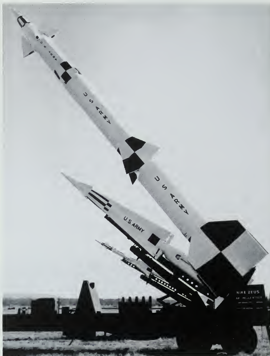
Fig. 2-3. The NIKE Family of missiles. From back to front: NIKE-AJAX, NIKE-HERCULES and NIKE-ZEUS.
